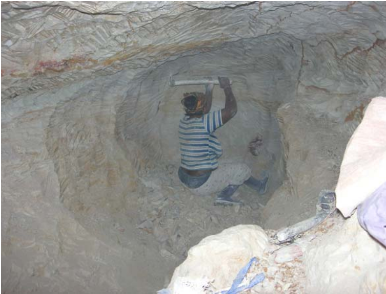
Figure 6: Ndwedwe – mining kaolin underground. Note the normal clothing and lack of head protection
